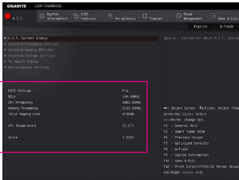
This section provides information on the BIOS version, CPU base clock, CPU frequency, memory frequency, total memory size, CPU temperature and CPU voltage, etc.
