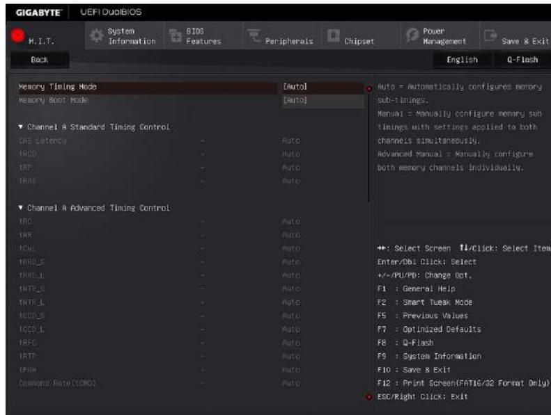
This sub-menu provides memory timing settings for each channel of memory. This sub-menu provides memory timing settings for each channel of memory. The respective timing setting screens are configurable only when **Memory Timing Mode** is set to **Manual** or **Advanced Manual**. Note: Your system may become unstable or fail to boot after you make changes on the memory timings. If this occurs, please reset the board to default values by loading optimized defaults or clearing the CMOS values.
